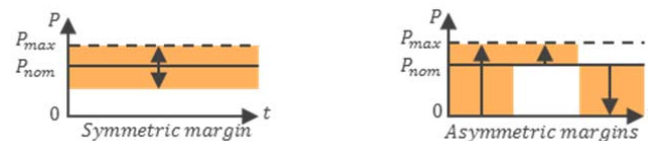
Figure 50: Symmetric and asymmetric frequency reserve participation principle schemes
